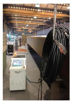
Demagnetization of a steel box girder
