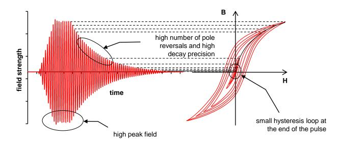
The following pulse parameters were identified in practical experiments and are preferably used for demagnetization of large surface steel objects (up to ~60mm wall thickness):
