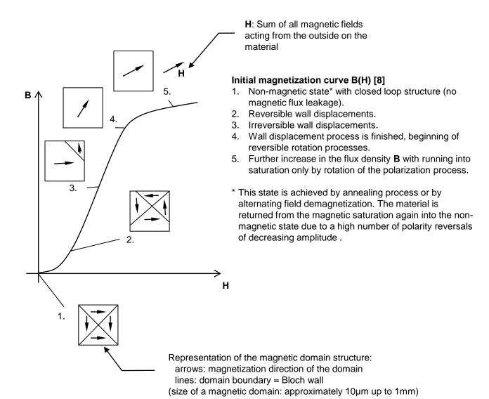
The Reversing Field, Knockdown and Demagnetization procedures described below reference to the initial magnetization curve.
