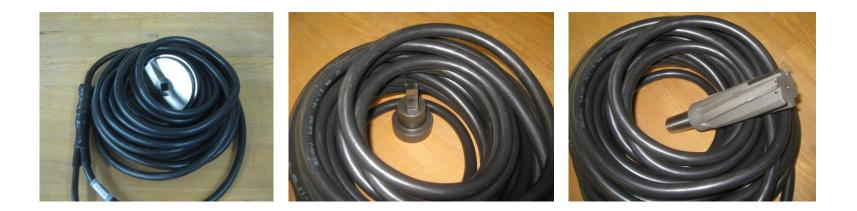
Demagnetization of materials with high coercivity (tungsten carbide, high-strength tool steels etc.) with power module DM200 and cable coil K10/2.5-15:
