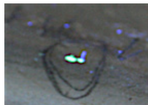
Fluorescent Penetrant Indication on Aluminum Extrusion
