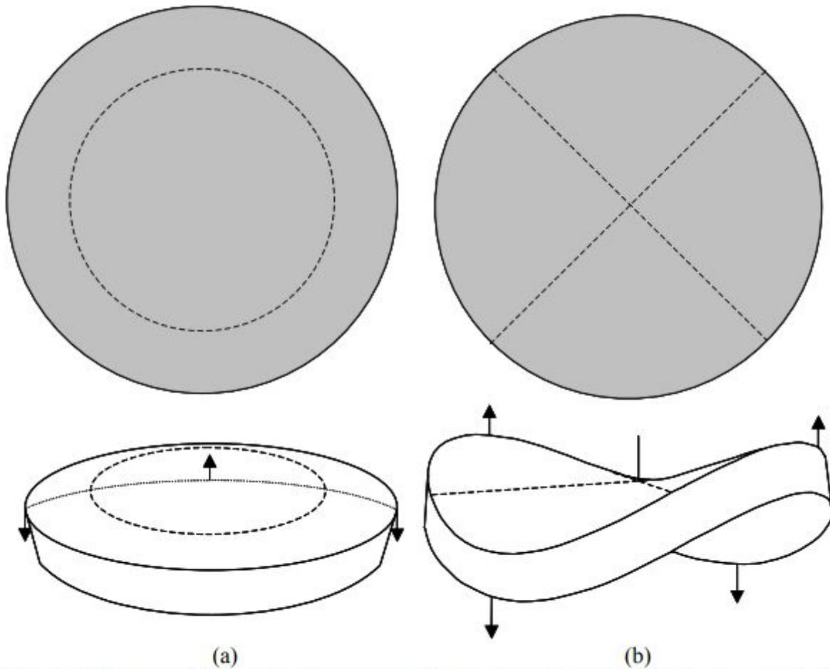
**Figure 22:** The first two modes of vibration of a disc, (a) flexural or 'diaphragm' mode, (b) torsional or 'saddle' mode. The dashed lines indicate the nodal lines and the arrows the direction of motion.
