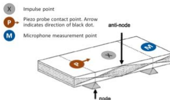
**Figure 23a:** supporting and exciting principal flexural resonance mode
