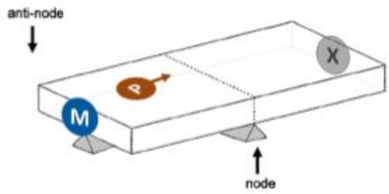
**Figure 23b:** Supporting and exciting principal torsional resonance mode
