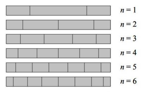
Figure 20: Out-of-plane vibration modes of a 'free-free' beam with the nodal lines indicated
