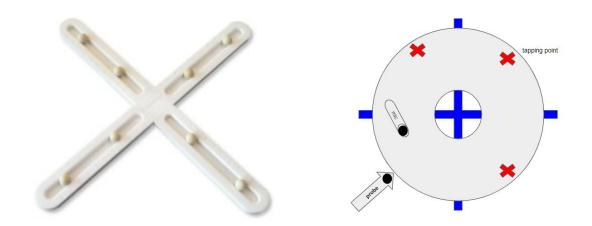
Figure 23c: Support and excitation of grinding wheel
