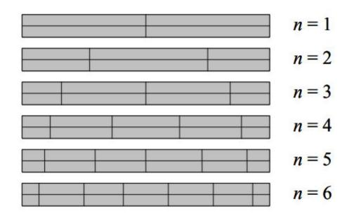
Figure 21: Torsional vibration modes of a 'free-free' beam with the nodal lines indicated.
