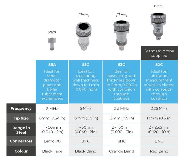
All probes need to be used with Ultrasonic Couplant when taking measurements (excl. underwater)
