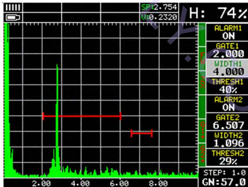
Centerline crack, note complete loss of Back Wall Echo
