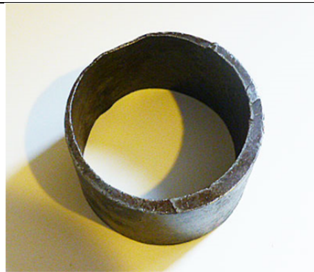
Figure 17 Severe Eroded Pipe Wall
