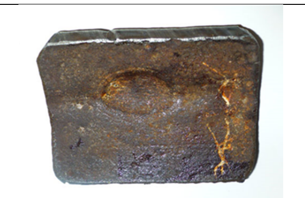
Figure 15 Severe Lake Shaped Pitting
