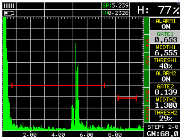
Cracked Pin – 2 nd Zone Crack
