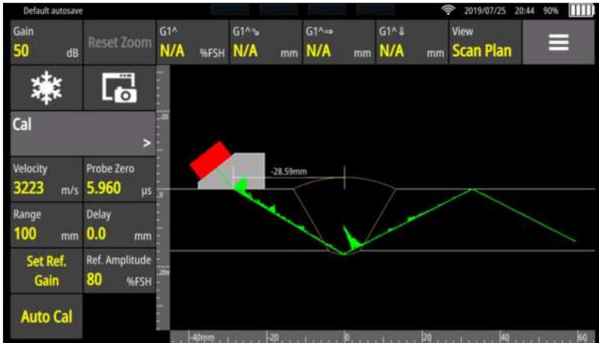
Geometrical indication at the root of the weld sample
