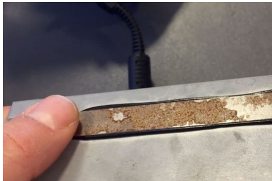
Two 0.8mm steel plates glued together
