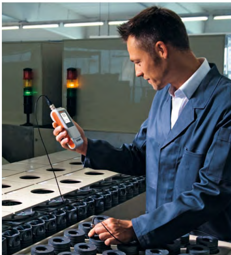
Quality monitoring on engine pistons immediately after the manufacturing process using the FIA3.3H probe
