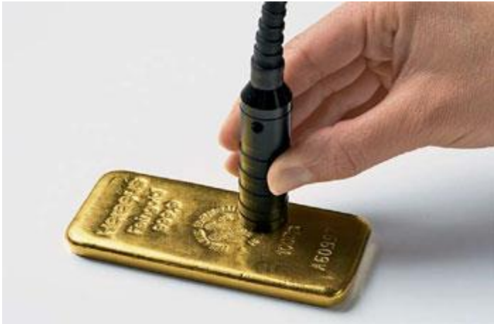
Testing of a fine gold bullion – even under plastic cover
