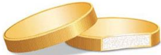
Counterfeit coins – filled with another metal hidden by a thin outer layer of the original material.
