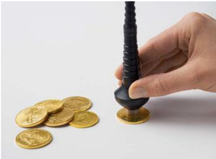
Testing for counterfeit coins – eddy current method
