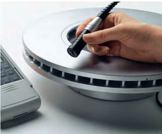
Measurement of zinc powder coating with the two-pole probe V7FKB4
