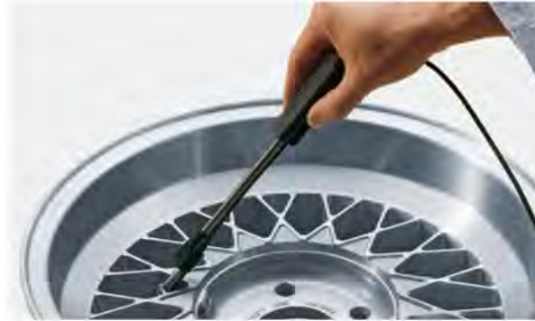
Measurement of the lacquer thickness on an aluminum rim wheel with the probe FAW3.3, mounted in the guiding device
