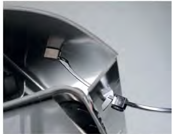
Auto body in section to show how the probe measures the EPD coating within the auto body
