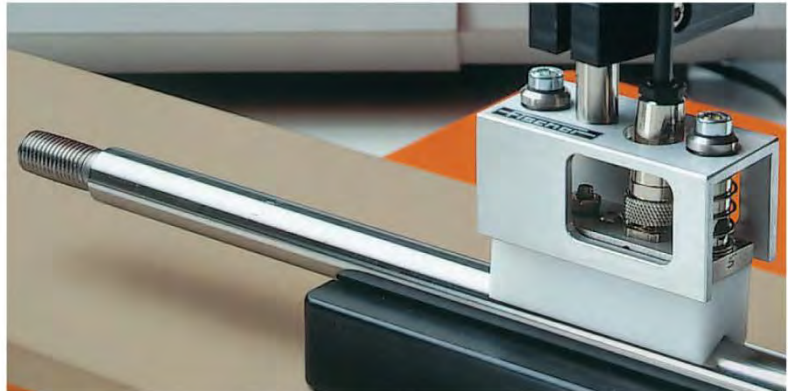
Automated measurement of the chrome coating on piston rods with the probe V2EGA06H
