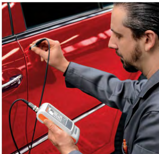
Measurement of auto body paint thickness using the Dual probe FD10
