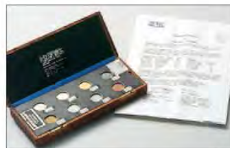
Internationally recognized Boeing Standards are used to establish the working standards of the SIGMASCOPE® SMP10
