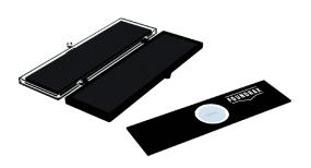
A Foundrax Stage Micrometer (a certified checking scale) can be supplied as an optional extra and provision is made for it in the microscope case.
