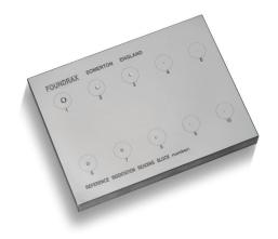
These are steel blocks containing 5 reference indentations made with a 10mm ball in the range 2.40-6.00mm and 5 reference indentions made with a 5mm ball in the range 1.20-3.00mm. These measuring ranges cover all Brinell scales using 10mm and 5mm Brinell balls.
