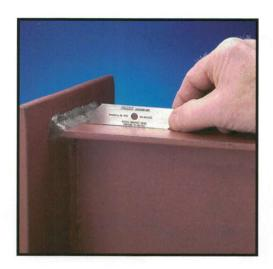
Undercut shall be no more than .010 in. (0.25) mm) deep when the weld is transverse to the primary stress in the part that is undercut.
