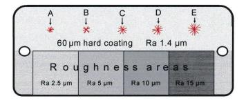
The ISO Panel is made from a 2.5 mm (0.1") stainless steel plate. Half of the test surface is 60 µm (0.0024") hard coated. Five crack centers are evenly spaced in the hard coated strip. The crack centers are circular patterns forming a star.
