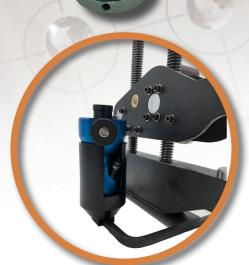
**Mew** Microscope stand for convenient and easy access. The stand can attach to any of our portable Brinell tester bases or be used as a stand alone.
