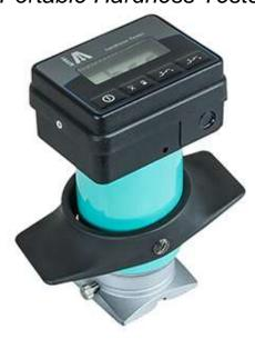
The **METALTEST** is a compact, pocket-sized, wireless hardness tester with commands and LCD incorporated on the top. It is very easy to use. Place the hardness tester on the surface to be examined and press the handgrip right down, release the pressure and the hardness immediately appears on the display.
