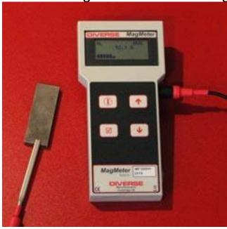
The Diverse MF300H+ hand-held battery operated Magnetic Field Meter, with its rugged stainless-steel Hall effect probe, is suitable for laboratory and workshop use.
