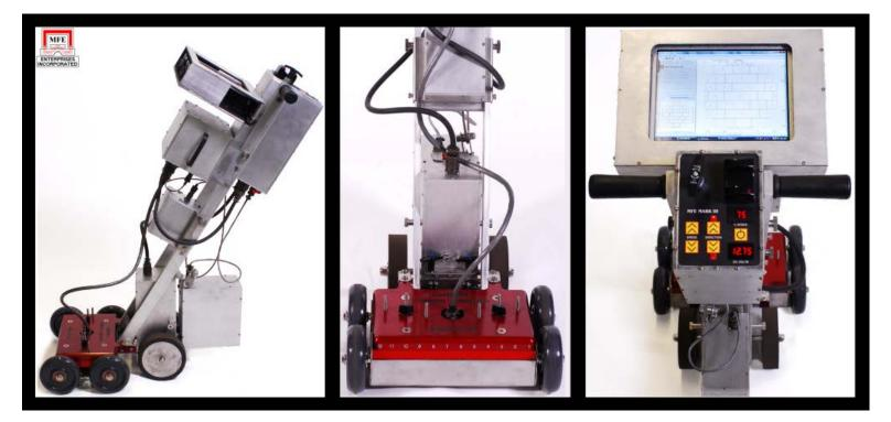
THE MARK III SERIES OFFERS IMPROVED INSPECTION RESULTS THROUGH COATED FLOORS AND THICKER PLATES, FULLY ADJUSTABLE LIMITS FOR ENHANCED THRESHOLDING TECHNIQUES, AND THE ABILITY TO PRODUCE COLOR-CODED MAPS OF CARBON STEEL LOSS ACROSS TANK FLOORS.
