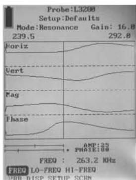
Real Time Reference Presentation. Displays X, Y, Phase & Amplitude
