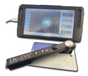
The UV-EYE is a must have tool for all Level III's and many other inspectors doing Fluorescent LPI, MPI and Visual inspections. It allows you to measure and record indications and send them to your computer for test reports and side by side comparisons of TAM indications.
