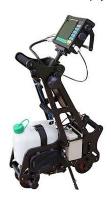
The USDS2-77-BASIC is a simplified version of the UDS-2-77-AREMA. It has 5 probes: 2-45\* degree, 2-70 degree and one 0 degree probe as shown below
