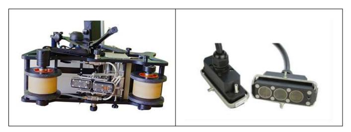
UDS2-77-BASIC ultrasonic rail flaw detector is intended for defect detection in rail along the running surface and rail cross-section, except for the rail foot flanges. It can also be used for manual check testing of welded joints and evaluation of detected defects. Test results are stored in non-volatile memory.
