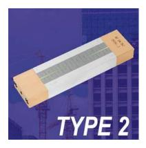
**Reference Block Type 2** consists of a steel bar with a scale machined into its face with 2 permanent magnets on either end. The scale is calibrated such that the +4 mark represents a magnetic field with a strength of +100 A/m and the -4 mark represents -100 A/m.
