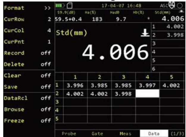
Measurements are recorded and displayed in grids.
