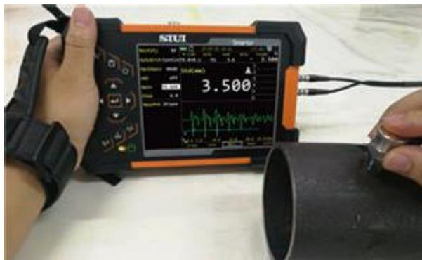
Thickness measurement on pipe
