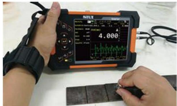
Thickness measurement on step block
