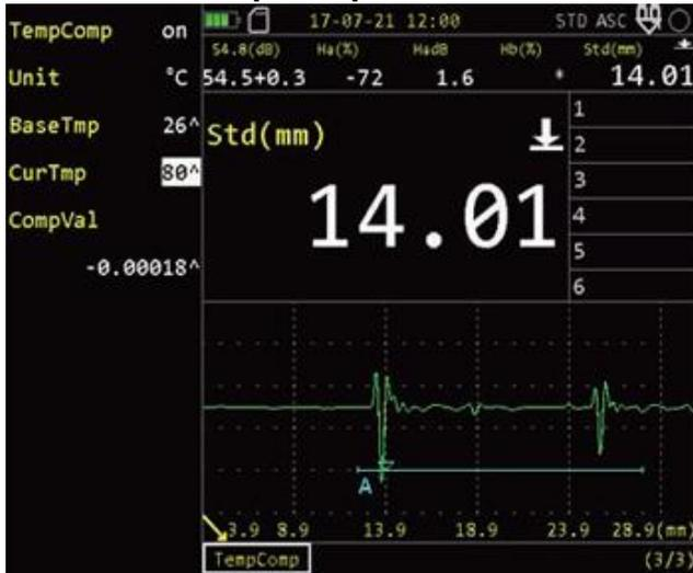
When there is a temperature difference between the calibration block and the detected workpiece, this can be used for temperature compensation.
