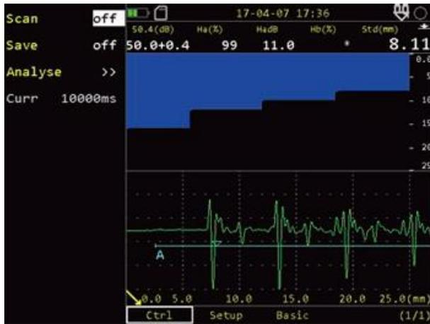
Based on time interval or encoder, you can display the measurement readings in a B-mode image.
