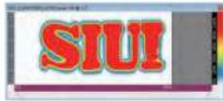
C Scan In-Amplitude, showing echo amplitude
