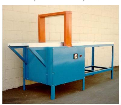
NOTES: The track and carriage reduces the use-able height of the coil opening By 2 1/4".
