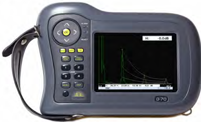
Masterscan D-70 DAC Curve functionality shown in Full Screen Mode.
