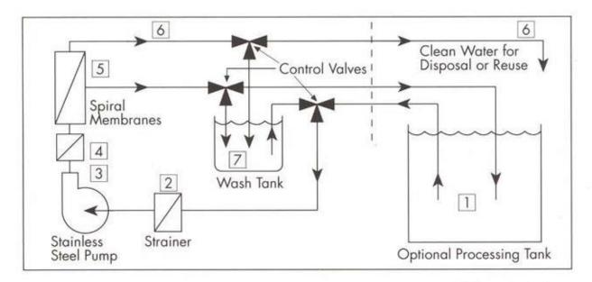
Oily wastewater is drawn from the processing tank 1 and fed to the strainer 2 for removal of large solid particles. From there, the stainless steel pump 3 transports the wastewater under pressure to the prefilter 4 and spiral membranes 5. Here the clean water 6 is separated for discharge or reuse while the oily wastewater is re-circulated to the processing tank. The three control valves can be adjusted to re-circulate detergent from the on-board wash tank 7 for periodic membrane cleanings.
