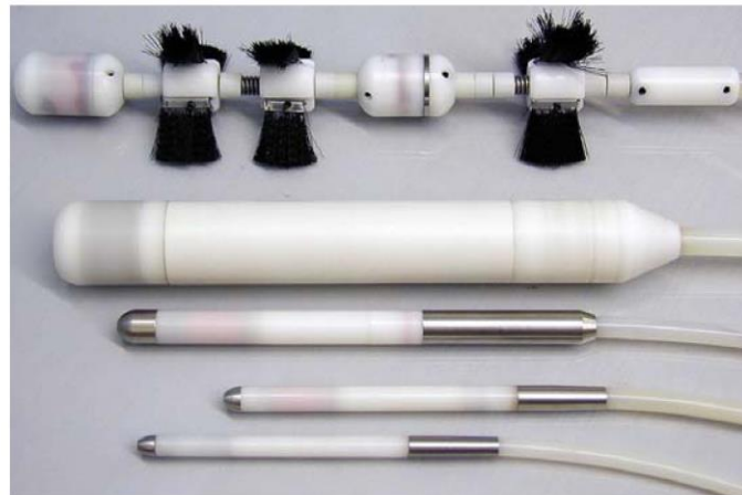
Assortment of various rigid and flexible RFET probe styles and sizes
