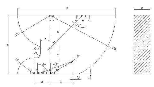
The V-3 Calibration Block for calibrating ultrasonic flaw detection equipment in both laboratory and on-site conditions. This block is intended to function as a more compact and light-weight alternative to V1 or IIW-Type Test Blocks. Includes 25mm, 50mm, and 100mm radii, (2) 3.0mm diameter through holes, engraved reference mark scales, and a 0.4mm wide x 2.5mm deep slot.
