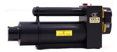
The XRS-4 is a 370kV, battery operated, pulsed X-ray generator used in security and light industrial applications. Pulsed X-rays generate a high intensity X-ray energy burst (pulse) in a very short period of time (10 nanoseconds). The XRS-4 provides a significant increase in penetrating capabilities compared to other models, 1.5" of steel when used with a digital imaging system. The output dose of each pulse is approximately 5mR measured 12 inches from the X-ray machine.
