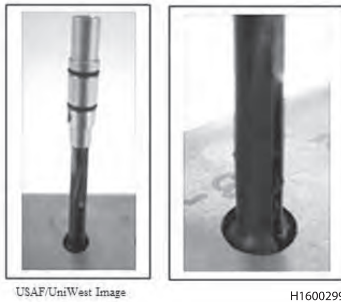
Figure 4-36. Checking Probe Fit
