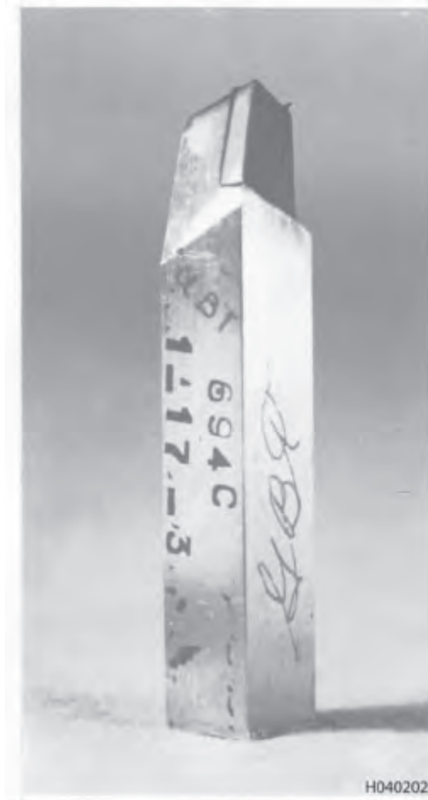
Figure 3-44. Magnetic Particle Indication of the Braze Line of a Brazed Tool Bit
