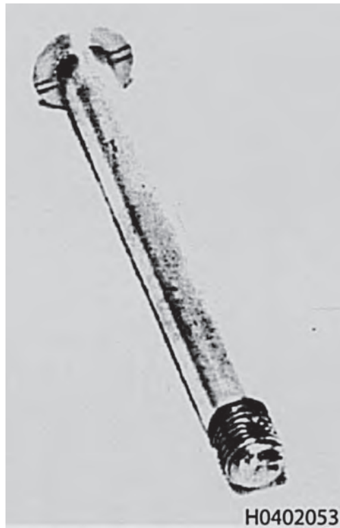
Figure 3-71. Non-Relevant Indications Under the Head Created by Slot in Bolt
