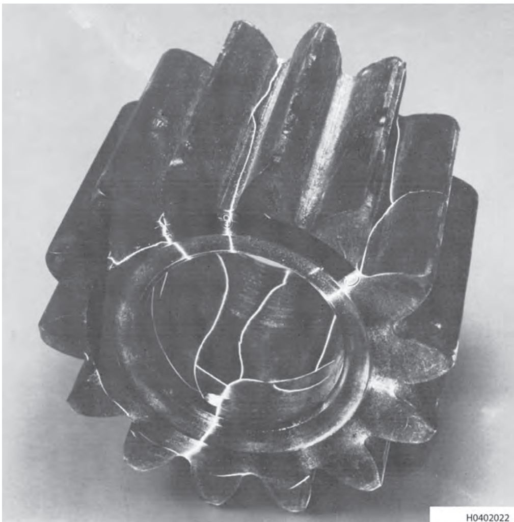
Figure 3-41. Typical Magnetic Particle Indications of Cracks
