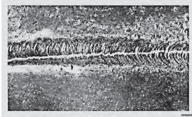
Figure 3-39. Sharp, Well Defined Indication of Surface Discontinuity in a Weld
