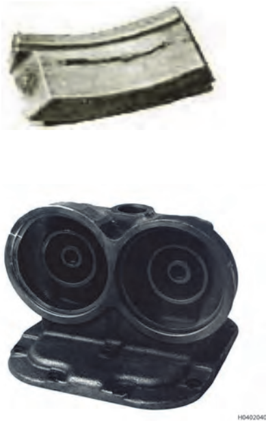
Figure 3-59. Magnetic Particle Indications of Defects in Castings
