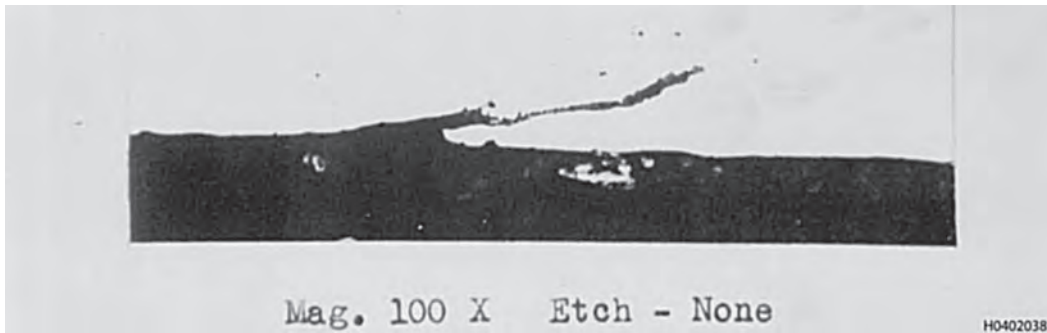
Figure 3-57. Cross Section of a Forging Lap (Magnified 100X)
