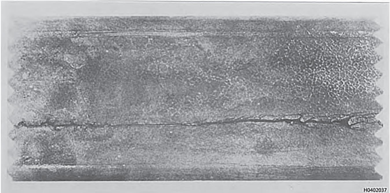
Figure 3-56. Surface of a Steel Billet Showing a Lap
