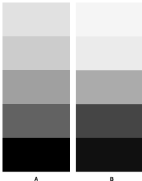
Figure 22: A: 220 kV exposure. B: 120 kV exposure. Radiographs of steel stepped wedge having a thickness range of 1/4 to 3/4 inch in 1/8-inch steps.
