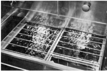
Figure 74: Water should flow over the tops of the hangers in the washing compartment. This avoids streaking due to contamination of the developer when hangers are used over again.
